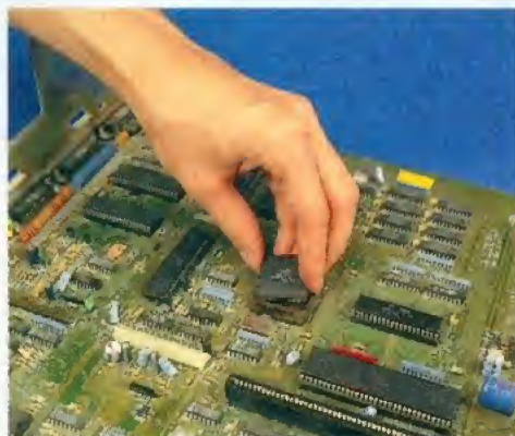
6 Remove the Agnus (preferably with the correct tool) and note the orientation. Then slip in the Megachip2 board, pushing home firmly.
